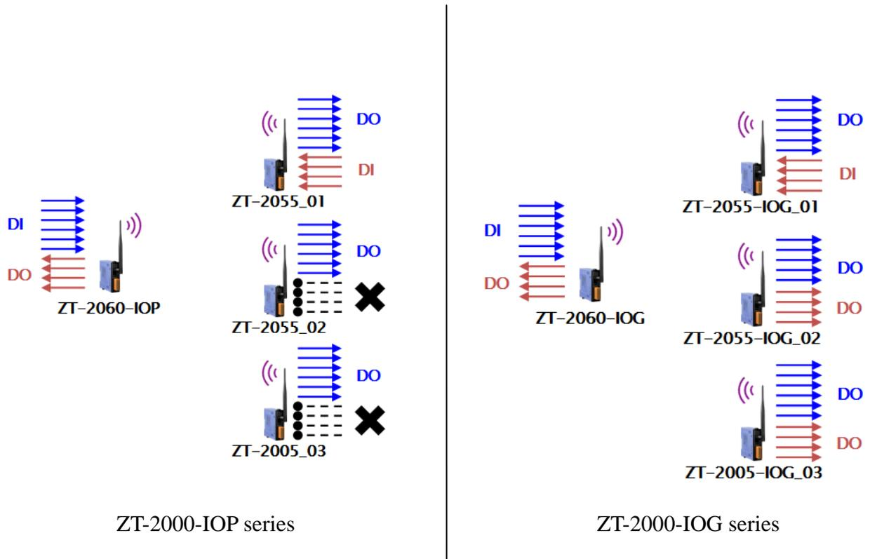
Fig.3-1. The different between ZT-2000-IOP and ZT-2000-IOG
