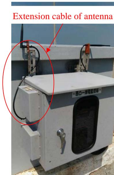
Fig. 2-2 Use extension cable of antenna
