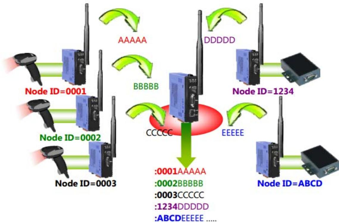
Fig5-1. Architecture of non-addressable device
