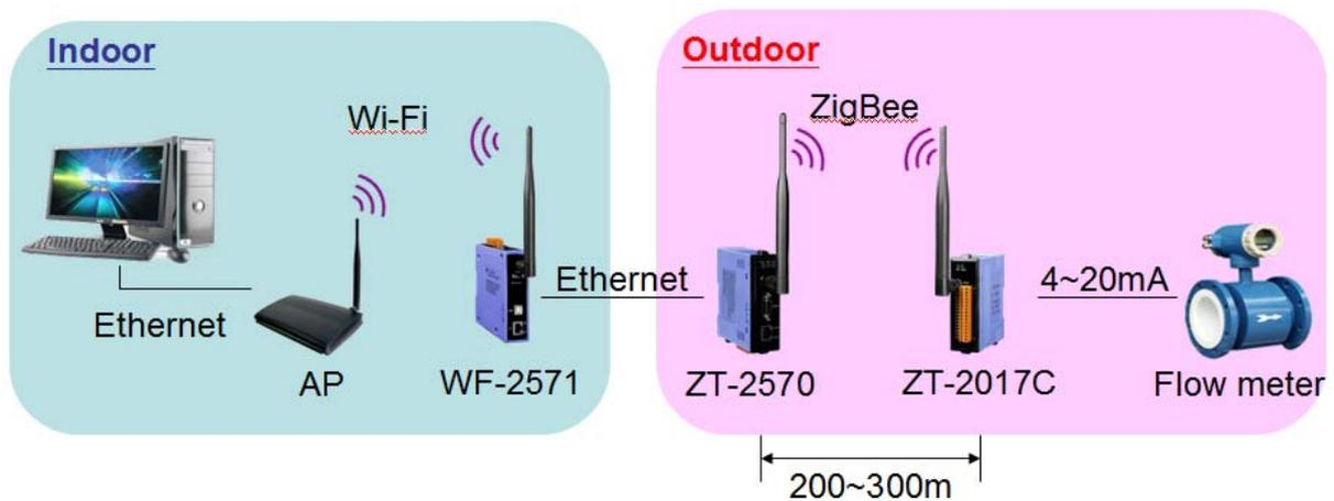
Fig. 3-1 Application architecture diagram of Wi-Fi to ZigBee
