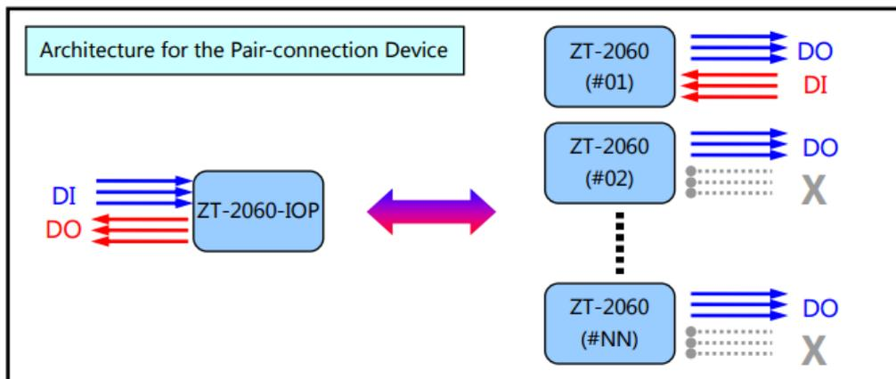
Fig3-1.Pair-connection of ZT-2000-IOP series
