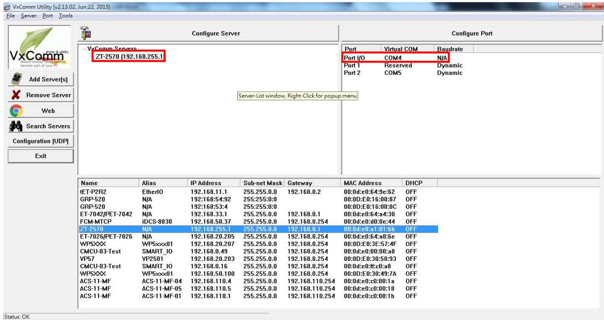
Fig-1-3. Setting virtual COM port of ZT-257x
