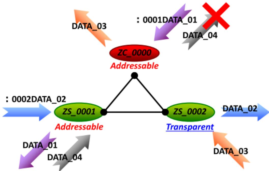
**Q4 · When the data was send to the RS-232 / RS-485 / Ethernet of the ZigBee converter (ZT-255x/ZT-257x) at the same time, how will the ZigBee converter dealt with the data? (2013/09/23, Bao)**
